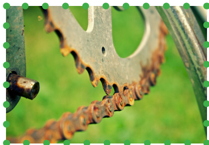
Rust is a chemical reaction of iron, water and oxygen.
